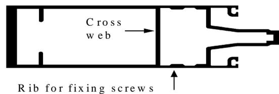
**Figure 1** Section of typical curtain walling mullion
